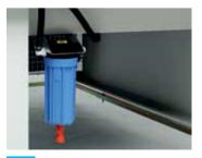
The filter house is conveniently mounted under the frame, allowing access to the cooling unit and extra storage space.
