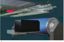
While the current plate is being exposed, the plate scheduled to be exposed next is punched and then moved to the standby cassette's upper tray.
