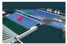
4 While the plate is being exposed, the plate scheduled to be exposed next is punched and then moved to the standby cassette's upper tray. The plate that was just exposed is transferred from the standby cassette's lower tray to the automatic inline developer.
