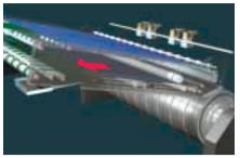
2 The plate that was just exposed is transferred to the standby cassette's lower tray.
